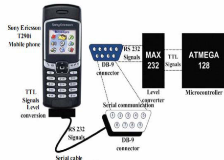
Figure 3: Serial Communication and Level Conversion between T290i and MCU
