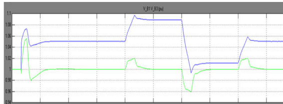
Fig 13: Voltage Wave form at Bus 1 & Bus 3 (pu)
