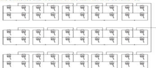
Fig. 1. Eleven-level cascaded multilevel STATCOM.
