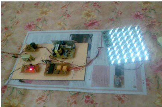
Fig. 6 Photo of lighting the LEDs, that are utilizing the proposed driver for lightening of the 88W of LEDs by selecting 110V output supply from LED driver
